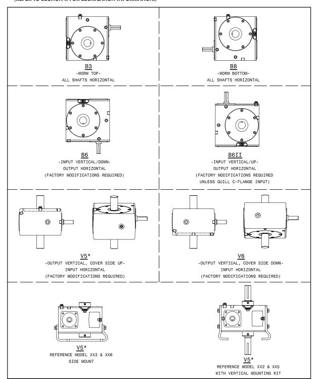
\* V5 IS THE PREFERRED MOUNTING POSITION FOR VERTICAL OUTPUT FACTORY MODIFICATIONS NOT REQUIRED WITH HIGH OIL LEVEL. SINGLE REDUCTION
